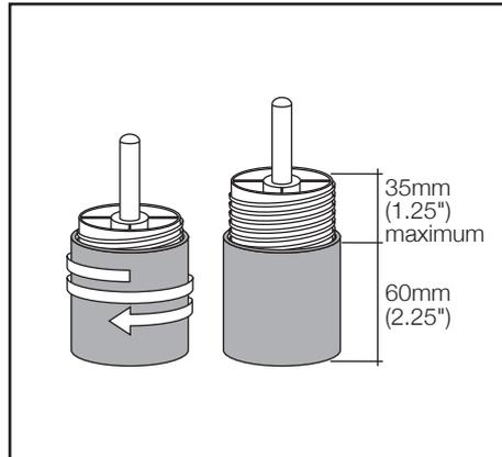
2. Adjustable Legs to keep bed level on uneven surfaces.
